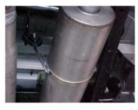
SLIDE BAND CLAMP #G ONTO MUFFLER #B. INSERT HANGERS INTO RUBBER GROMMETS. SUGGESTED TOOLS:
