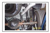
Install the over axle tailpipe # C into the muffler 1-1/2" to 2". Secure to the muffler using clamp # F Do not tighten.
