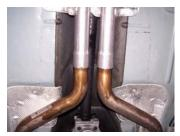
Lay out the exhaust on the floor so it looks like the drawing and compare parts with manual. To remove the stock exhaust, first you must remove the crossmember under the X-pipe. Then unbolt and remove driver side tailpipe at the flange. Now unbolt and cut tack welds on factory clamps at the X-pipe and carefully remove factory exhaust, save clamps for new exhaust installation. Leave all rubber grommets on hangers. Use WD-40 to help remove hangers.
