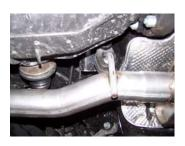
Install driver side tailpipe/muffler assembly #B. Insert all welded hangers into rubber grommets. Secure tailpipes with clamp #D. Do not tighten.
