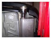
**5.** Adjust assembly to fit to your liking. When you have everything in place, firmly tighten all bolts and clamps down securely. Use stainless steel cleaner and a Scotch Brite pad weekly to prevent tip from discoloration.
