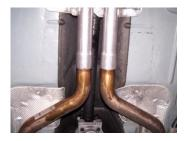
2. To remove the stock exhaust, first you must remove the factory cross member under the X pipe. Then unbolt and remove driver side tailpipe at the flange. Now unbolt and cut tack welds on factory clamps at the X pipe and carefully remove factory exhaust, save clamps for new exhaust installation. Leave all rubber grommets on hangers. Use WD-40 to help remove hangers.
