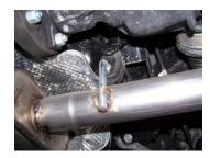
Install passenger side tailpipe assembly #C. Insert all welded hangers into rubber grommets. Secure tailpipe with clamp #D. Do not tighten.
