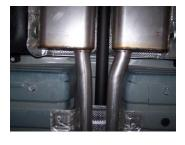
Install X-pipe assembly #A assembly on to your front factory pipes and secure with factory clamps. Reinstall factory cross member. Use a jack stand to support mufflers. Do not tighten.
