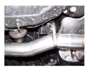
Install driver side tailpipe assembly #B. Insert all welded hangers into rubber grommets. Secure tailpipes with clamp #D. Do not tighten.
