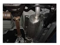
INSTALL MUFFLER #C 1-1/2" TO 2" ONTO THE HEADPIPE WITH INLET FACING TOWARDS THE MOTOR. ROTATE THE MUFFLER UNTIL THE OUTLET IS AT THE 2 O'CLOCK POSITION. USE CLAMP #F TO SECURE THE MUFFLER TO THE HEADPIPE. MUFFLER INLET IS LOOKING INTO THE LOUVERS. DO NOT TIGHTEN.
