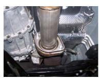
Install head pipe # A onto your existing stock flange and secure with bolt kit #G. DO NOT TIGHTEN.
