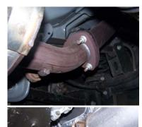
Lay out the exhaust on the floor so it looks like the drawing and compare parts with manual. Remove the stock exhaust from the 3 bolt flange just behind the muffler, then remove the back section, then the remaining stock exhaust from the 2 bolt flange in front of the muffler. Leave all rubber grommets in place. Use WD-40 to aid in removal of hangers.
