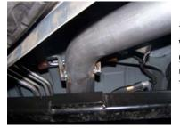
Install extension pipe #C into the muffler 1½-2". Insert welded hanger into rubber grommet. Secure the muffler using clamp #F. DO NOT TIGHTEN.
