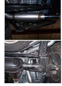
Install the over axle tail pipe w/welded resonator onto extension pipe, insert welded hangers into grommets and use clamp #F to secure pipes together. DO NOT TIGHTEN.
