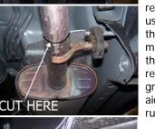
**1.** To remove the stock exhaust remove the nut on the rear hanger using a 21mm wrench, then cut the tailpipe just after the rear muffler hanger and remove. Unbolt the headpipe at the flange and remove. Leave all rubber grommets in place. Use WD-40 to aid in removal of hangers from rubber grommets.
