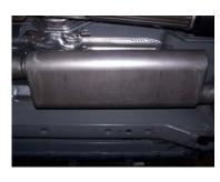
Install muffler #B onto head pipe #A 1½-2" with the louvers facing towards the converter. Use a jack stand to support the muffler. Use clamp #E to secure the muffler to the head pipe. DO NOT TIGHTEN. Muffler inlet is looking into the louvers.
