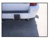
**5.** Install stainless steel tips. Clamp down. When you have everything in place, firmly tighten all bolts and clamps down securely. Use stainless steel cleaner and a Scotch Brite pad weekly to prevent tip from discoloration. Inspect all fasteners after 25-50 miles of operation and retighten as necessary.
