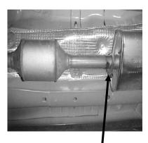
FOR EASIER REMOVAL OF THE FACTORY EXHAUST. CUT THE TAILPIPE BEHIND THE MUFFLER. THEN REMOVE THE FACTORY MUFFLER AT THE CLAMP IN FRONT OF THE MUFFLER. USE A JACK STAND TO SUPPORT THE CONVERTER ONCE EXHAUST IS REMOVED. NOTE LEAVE ALL FACTORY RUBBER GROMMETS IN PLACE
