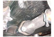
**INSTALL HEADPIPE #A** USING FLANGE #H AND HARDWARE KIT #F ONTO EXISITING FLANGE. DO NOT TIGHTEN.
