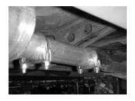
Install head pipe # A 1" to 1 ½" on to your existing stock front pipe and secure with clamp # G. Do not tighten.
