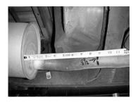
Lay out the exhaust on the floor so it looks like the drawing and compare parts with manual. To remove the stock exhaust cut 8 ½" inches in front of the muffler. Leave all rubber grommets in place. Use WD-40 to aid in removal of exhaust and hangers.
