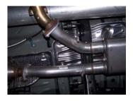
4. Install muffler onto headpipes 1.5"-2" with the louvers facing towards the converter. Use a jack stand to support the muffler. Use clamps #G to secure the muffler to the headpipe. Do not tighten. Muffler inlet is looking into the louvers.
