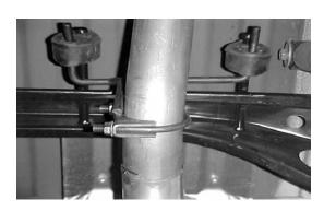
INSTALL REAR MUFFLER OE HANGER #F TO SUPPORT THE TAILPIPE.THE BOLTS FROM THE OE HANGER WILL BE FACING THE
