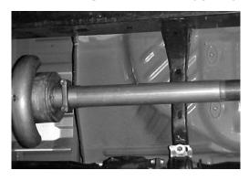
SLIDE THE HEADPIPE ONTO THE STOCK HEADPIPE USING CLAMP # E. THEN INSTALL THE MUFFLER ON HEADPIPE #A NO LESS THAN 1-1/2" TO 2" USING CLAMP #E. THE MUFFLER OUTLET WILL BE CLOCKED AT 12 O'CLOCK POSITION. INLET OF MUFFLER HAS LOUVERS FACING THE MOTOR. DO NOT TIGHTEN
