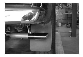
INSTALL THE STAINLESS TIP. USE A STAINLESS OR ALUMINUM CLEANER TO POLISH TIP. NOW TIGHTEN ALL HANGERS AND CLAMPS.
