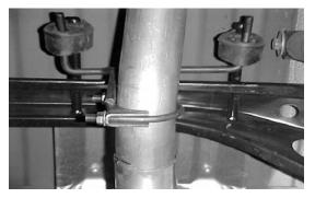
INSTALL REAR MUFFLER OE HANGER #F TO SUPPORT THE TAILPIPE.THE BOLTS FROM THE OE HANGER WILL BE FACING THE DRIVERSIDE. THIS HANGER ATTACHES TO THE TAILPIPE, NOT THE MUFFLER. DO NOT TIGHTEN.
