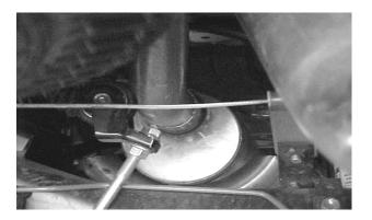
INSTALL OVERAXLE TAILPIPE # C INTO THE MUFFLER, USING CLAMP # E. INSERT WELDED HANGER INTO RUBBER GROMMET.
