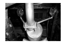
NEXT INSTALL REAR MUFFLER HANGER #G ONTO OUTLET OF MUFFLER. INSERT WELDED HANGER INTO RUBBER GROMMETS
