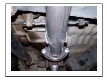
To remove the stock exhaust it, unbolt it at the flange just in front of the muffler and remove stock exhaust. Leave all rubber grommets in place. Use WD-40 to aid in removal of exhaust and hangers.
