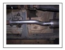
Attach head pipe # A on to your existing stock front pipe and secure with bolt kit # E. Use a jack stand to support the converter. Insert welded hanger into rubber grommet. Do not tighten.
