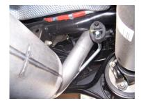
5. Install the over axle tailpipe #C into the muffler 1.5-2". Secure to the muffler using clamp #F. Do not tighten. Insert welded hanger into rubber grommet.
