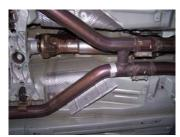
2. Loosen up the 2 clamps in the middle of the vehicle and slide them over the tailpipes.
