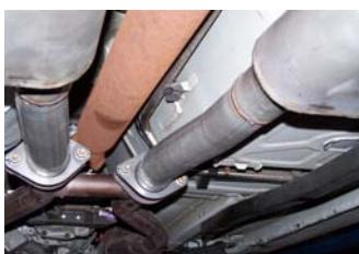
3. Install head pipes #A & B onto your existing stock front pipe and attach with factory hardware. Do not tighten.
