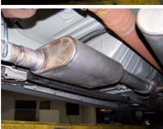
5. Install drivers side overaxle tailpipe #E into mufflers 1 1/2" to 2". Insert welded hangers into rubber grommets use clamp #I to secure to muffler. Do not tighten.
