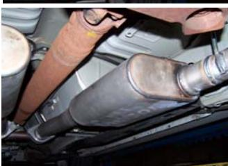
4. Install mufflers #C onto head pipes 1 1/2"-2" with the louvers facing towards the converter. Use a jack stand to support the muffler. Use clamps #I to secure the muffler to the headpipe. DO NOT TIGHTEN. Muffler inlet is looking into the louvers.
