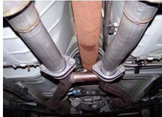
2. To remove the stock exhaust, remove it from the 2 bolt flanges located in front of your factory mufflers. Disengage the welded hangers using WD-40 from the OEM rubber grommets. Do not damage or remove the rubber grommets as you will reuse them to mount your new system. Now, cut off tailpipes before and after rear axle for removal.
