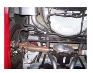
6. Now do the same procedure for the driver side tailpipe. Use clamp #E to secure the tailpipe to the muffler assembly and the stock clamp to secure it to the stock h-pipe.
