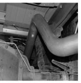
INSTALL TURNOUT PIPE #D TO THE OVERAXLE TAILPIPE. ROTATE PIPE SO IT IS AT THE CORRECT ANGLE FOR YOUR VEHICLE. USE CLAMP #G TO ATTACH.
