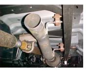
Install head pipe # A on to your existing stock front pipe and line up the notch. Then secure with clamp # H. Insert hangers into rubber grommets. Do not tighten.
