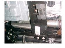
INSTALL PIPE #K ONTO PIPE #J. USE CLAMP #H. TO SECURE PIPES TOGETHER. DO NOT TIGHTEN.
