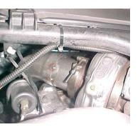
REMOVE THE REMAINING STOCK DOWN PIPE BY **UNCLAMPING IT FROM** THE TURBO HOUSING. USE A 11MM SOCKET OR WRENCH TO REMOVE YOUR STOCK PIPE THROUGH THE BOTTOM. DO NOT DISGARD THE STOCK CLAMP YOU WILL NEED TO RE-USE IT.
