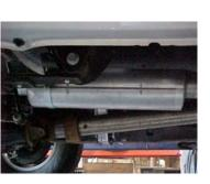
Install muffler # B onto head pipe # A 1-1/2" to 2" with the louvers facing towards the converter. Use a jack stand to support the muffler. Use clamp # G to secure the muffler to the head pipe. Do not tighten. Muffler inlet is looking into the louvers.
