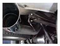
Install exit pipe # D onto overaxle pipe. Then insert welded hanger into rubber grommet. Use clamp # G to secure pipes together.
