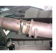
TO INSTALL YOUR GIBSON DOWN PIPE YOU NEED TO REMOVE YOUR STOCK EXHAUST. REMOVE THE STOCK EXHAUST FROM THE **CLAMP LOCATED JUST** BEHIND THE CATALYTIC CONVERTER. CUT OFF YOUR STOCK TAILPIPE FOR EASIER REMOVAL. LEAVE ALL RUBBER GROMMETS IN PLACE. USE WD-40 TO AID IN REMOVAL OF EXHAUST AND HANGER. AFTER YOUR STOCK EXHAUST IS REMOVED YOU NEED TO REMOVE THE CATALYTIC CONVERTER FROM THE 2-BOLT FLANGE.
