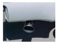
Install stainless steel tip. Clamp down. When you have everything in place, firmly tighten all bolts and clamp down securely starting from the Turbo and work your way back to the rear of the vehicle. To clean stainless steel tip use any stainless steel cleaner and Scotch Brite pad.
