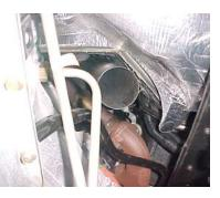
INSTALL PIPE #J ONTO TURBO USING YOUR STOCK CLAMP. DO NOT TIGHTEN.
