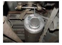
INSTALL MUFFLER #B ONTO HEADPIPE #A 1-1/2" TO 2". USE A JACKSTAND TO SUPPORT MUFFLER. SECURE MUFFLER TO HEADPIPE WITH CLAMP #1. DO NOT TIGHTEN. INSTALL HANGER #G ONTO OUTLET OF MUFFLER AND INSERT HANGERS INTO RUBBER GROMMETS. MUFFLER INLET IS LOOKING INTO THE LOUVERS.
