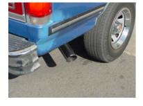
INSTALL THE STAINLESS TIP. TO CLEAN TIP USE ANY STAINLESS CLEANER AND A SCOTCH BRITE PAD. NOW GO BACK AND TGHTEN ALL CLAMPS STARTING FROM THE FRONT AND WORKING BACK.
