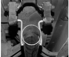
**UN-BOLT STOCK HEADPIPE** JUST BEHIND THE CATALYTIC CONVERTER. **DO NOT DAMAGE** STOCK BOLTS AND **GASKET! FOR YOU** WILL NEED TO RE-USE THEM. CUT OFF YOUR STOCK TAILPIPE JUST BEHIND THE MUFFLER AND REMOVE. LEAVE ALL RUBBER GROMMETS ON THE HANGER. USE WD-40 TO HELP WITH REMOVAL OF STOCK EXHAUST AND HANGERS.
