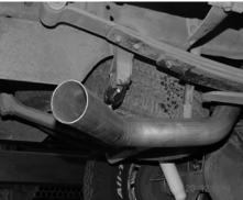
INSTALL TURNOUT PIPF # D ONTO OVERAXLE TAILPIPE USING CLAMP # E. **INSERT WELDED** HANGER INTO RUBBER GROMMET. DO NOT TIGHTEN.
