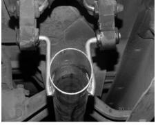
BOLT HEADPIPE # A TO THE STOCK FLANGE **RE-USING STOCK BOLTS** AND GASKET. INSERT WELDED HANGERS INTO RUBBER GROMMETS. DO NOT TIGHTEN.
