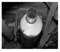
**INSTALL MUFFLER # B** INTO HEADPIPE AT LEAST 1-1/2" TO 2". USE CLAMP # E TO ATTACH TO THE HEADPIPE. USE A JACKSTAND TO SUPPORT THF MUFFLFR. DO NOT TIGHTEN.
