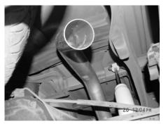
INSTALL OVERAXLE TAILPIPE # C INTO MUFFLER AT LEAST 1-1/2" TO 2" USING CLAMP #E TO ATTACH IT TO THE MUFFLER. DO NOT
