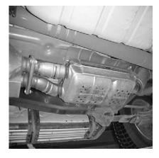
LAYOUT THE GIBSON EXHAUST AND COMPARE PART NUMBERS TO THE PIPE NUMBERS. FOR EASY REMOVAL, CUT THE STOCK TAILPIPE BEHIND THE MUFFLER AND ALSO BEHIND THE AXLE. NOW UNBOLT THE STOCK FLANGE AND REMOVE THE STOCK MUFFLER. DO NOT DAMAGE THE FACTORY GASKET BECAUSE YOU WILL RE-USE IT.
