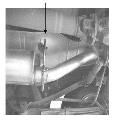
NEXT, INSTALL REAR MUFFLER HANGER #D AND INSERT INTO RUBBER GROMMETT. DO NOT TIGHTEN.
