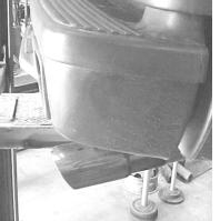
MAKE SURE YOU HAVE AT LEAST A 1" CLEARANCE ON ALL PIPES, RUBBER BRAKE LINES, FUEL LINES, SHOCK BOOTS, TIRES, ETC.
