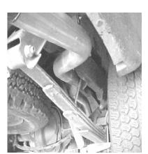
**INSTALL OVERAXLE** TAILPIPE #B AND ATTACH TO MUFFLER OUTLET USING HANGER **#D, WHEN INSTALLING** THE TAILPIPE YOU WILL NEED TO JACK THE BODY OF THE VEHICLE UP, TO SLIDE THE TAILPIPE THROUGH THE LEAF SPRING AND THE BOTTOM OF THE FRAME. ALSO THE SHOCK IN FRONT OF THE AXLE MAY NEED TO BE DISCONNECTED AND LOWERED TO SLIP THE TAIL PIPE IN. INSERT THE WELDED HANGER INTO THE RUBBER GROMMETT.
