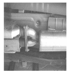
INSTALL MUFFLER ASSEMBLY ONTO THE STOCK FLANGE REUSING THE FACTORY GASKET AND HEADPIPE BOLT KIT #E. DO NOT TIGHTEN!!
