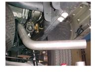
Install the turnout pipe #D on the tailpipe. Secure together with clamp #E. Do not tighten. Roll the exit pipe until it is at the correct angle for your truck. Insert welded hanger into rubber grommet.
