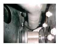
Install the over axle tailpipe #C into the muffler 1-1/2" to 2", and attach to hanger # F. Do not tighten down.
