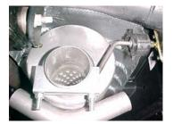
Install muffler #B onto head pipe 1-1/2" to 2" with the louvers facing towards the converter. Outlet will be at the 6 o'clock position. Use a jack stand to support the muffler. Use clamp #E to secure the muffler to the head pipe. Do not tighten. Muffler inlet is looking into the louvers. Next, install rear muffler hanger #F onto muffler outlet. Insert hanger into rubber grommet.
