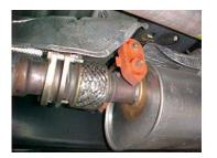
Lay out the exhaust on the floor so it looks like the drawing and compare parts with manual. To remove the stock exhaust Remove from the 2-bolt flange in front of your stock muffler. Also remove exit pipe from the clamp at the rear. Leave all rubber grommets in place. Use WD-40 to aid in removal of exhaust and hangers. Do not discard your factory hardware, for you will re-use it.
