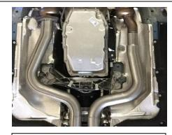
2. Install the PS headpipe Item A and Item B onto the factory pipes. Reuse the factory gaskets and hardware. Do not tighten. Keep loose until final fitment. Install O2 sensor at the end of the install.
