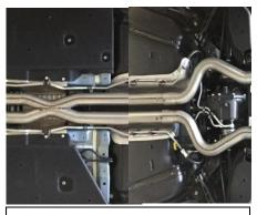
3. Install Item C onto the headpipes using clamps Item I to secure. Do not tighten. Install Item D & E onto the X pipe. Keep everything loose.
