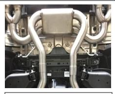
4. Install Item F onto the mid pipes. With everything kept loose it should slide on simply. Use a jack stand to support the muffler assembly and re install the factory hangers if you chose to un bolt them during the removal of the factory exhaust.
