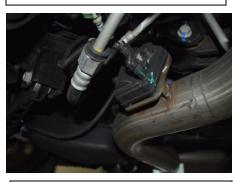
7. Remove the NPT valves from your factyory exhaust located on the tailpipes. Using your 10MM, install both onto your mid pipes and re connect. Re install your Factory 02 sensor. It may take 4-500 miles for your vehicle to fully adjust to the changes in exhaust flow.
