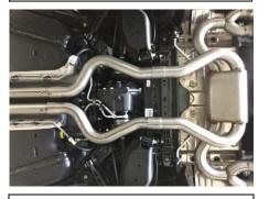
6. With a proper 1" clearance from all frame all pipes begin to tighten down all clamp connections from the front head pipe back. After each section has been tightened go back and re check all components for clearance.
