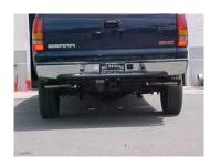
Install exit pipes #F. Use clamps #I to attach to tailpipes. These clamps also attach to the metal hangers # J. Rotate to adjust for clamping. Now go back and tighten up all clamps, nuts, and bolts.
