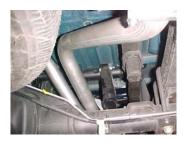
Install passenger side overaxle tailpipe #D into muffler 1 ½" to 2". Secure to muffler with clamp #I. Do not tighten. Next rotate pipe until it connects to rear hanger #J. Use clamp #J to hold up pipe.
