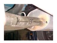
Lay out the exhaust on the floor so it looks like the drawing and compare parts with manual. To remove the stock exhaust cut 13" just in front of the muffler. Leave all rubber grommets in place. Use WD-40 to aid in removal of exhaust and hangers. Use hacksaw to cut tailpipe off.
