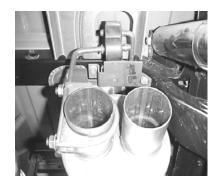
MEASURE 22" FROM THE REAROF THE FRAME. INSTALL TAILPIPE HANGER # G USING HARDWARE PROVIDED.
