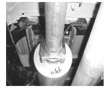
INSTALL MUFFLER ONTO STOCK HEADPIPE AND ATTACH WITH FRONT MUFFLER HANGER # I AND INSERT INTO RUBBER GROMMETS. ALIGN NOTCH ON GIBSON MUFFLER TO STOCK ALIGNMENT PIN ON FACTORY HEADPIPE. MUFFLER INLET IS TOWARDS THE CONVERTER .USE A JACK STAND TO SUPPORT THE MUFFLER.
