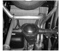
INSTALL PASSENGER SIDE OVERAXLE PIPE #D AND ATTACH TO MUFFLER USING CLAMP # F. INSERT HANGER INTO RUBBER.
