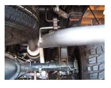
SLIDE PASSENGER SIDE TAILPIPE #E INTO MUFFLER 1-1/2" TO 2". USE CLAMP #I TO SECURE TAILPIPE TO MUFFLER. DO NOT TIGHTEN. INSERT HANGER INTO RUBBER GROMMET.
