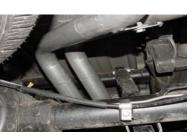
SLIDE PASSENGER SIDE TAILPIPE #E INTO MUFFLER 1-1/2" TO 2". USE CLAMP #I TO SECURE TAILPIPE TO MUFFLER. DO NOT TIGHTEN.
