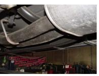
TO REMOVE STOCK EXHAUST, CUT 13" FROM THE FRONT OF THE MUFFLER, MEASURE TOWARDS THE FRONT OF THE VEHICLE. LEAVE ALL RUBBER GROMMETS ON THE HANGERS. USE WD-40 TO AID IN THE REMOVAL OF EXHAUST AND HANGERS. SUPPORT THE CATALITIC CONVERTER BEFORE CUTTING.
