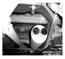
INSTALL MUFFLER #B ON TO THE HEADPIPE 1- 1/2" TO 2" WITH INLET TOWARDS CONVERTER USING CLAMP #G TO SECURE MUFFLER TO HEADPIPE. USE A JACKSTAND TO SUPPORT THE MUFFLER. DO NOT TIGHTEN.
