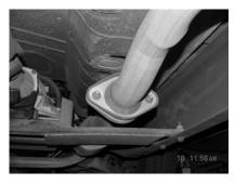
UNBOLT THE 2-BOLT FLANGE LOCATED BEHIND THE CONVERTER, SAVE STOCK NUTS AND BOLTS FOR YOU WILL REUSE THEM. NOW CUT OFF YOUR STOCK TAILPIPE JUST BEHIND THE MUFFLER AND REMOVE. USE WD-40 TO AID IN REMOVAL OF THE EXHAUST AND HANGERS. LEAVE ALL RUBBER GROMMETS ON THE HANGER. YOU NEED TO SUPPORT THE CONVERTER SO THE SYSTEM WILL NOT SIT ON THE CROSSMBMBER.
