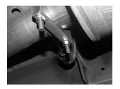
ADJUST MUFFLER ASSEMBLY. NOW TIGHTEN ALL BOLTS AND CLAMPS.
