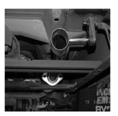
BOLT HEADPIPE #B TO STOCK FLANGE RE-USING STOCK NUTS AND BOLTS. INSERT WELDED HANGER INTO RUBBER GROMMETS.
