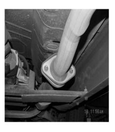
TO REMOVE EXHAUST- UNBOLT THE 2 BOLT FLANGE LOCATED BEHIND THE CATALITIC CONVERTER. SAVE STOCK NUTS AND BOLTS FOR YOU WILL REUSE THEM. NOW CUT OFF YOUR STOCK TAILPIPE JUST BEHIND THE MUFFLER AND REMOVE. LEAVE ALL RUBBER GROMMETS ON THE HANGER. USE WD-40 TO AID IN THE REMOVAL OF THE EXHAUST AND HANGERS.
