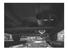
BOLT THE HEADPIPE #A ONTO FACTORY FLANGE USING GASKET #K AND RE-USING THE FACTORY NUTS AND BOLTS. SLIDE THE WELDED HANGER INTO THE RUBBER GROMMET. DO NOT TIGHTEN. INSTALL MUFFLER ON TO THE HEADPIPE 1- 1/2" TO 2" WITH INLET TOWARDS CONVERTER USING CLAMP **#F TO SECURE MUFFLER** TO HEADPIPE. USE A JACKSTAND TO SUPPORT THE MUFFLER. DO NOT TIGHTEN.
