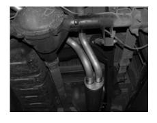
INSTALL PASSENGER SIDE TAILPIPE #C INTO MUFFLER 1-1/2" TO 2" USING CLAMP #G THIS WILL HOLD UP THE PIPE. ATTACH CLAMP #G TO TAILPIPE AND SECURE WITH HANGER #H.
