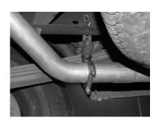
INSTALL EXIT PIPES #E ONTO TAILPIPES. ROLL EXIT PIPES UNTIL YOU HAVE THE CORRECT ANGLE. USE CLAMPS #G TO SECURE TO THE TAILPIPES. DO NOT TIGHTEN. CUT EXIT PIPE TO PROPER LENGTH.
