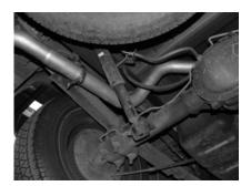
INSTALL DRIVERSIDE TAILPIPE #D INTO MUFFLER 1-1/2" TO 2". THIS PIPE GOES BETWEEN THE SHOCK & FRAME. SLIDE CLAMP #G OVER PIPE AND CONNECT IT TO THE HANGER#H. THIS WILL HOLD UP THE TAILPIPE. ATTACH TAILPIPE TO MUFFLER OUTLET USING CLAMP #I.
