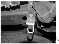
INSTALL METAL HANGERS #H INTO HOLES LOCATED APPROX. 16" FROM THE REAR OF THE FRAME. METAL HANGERS ARE MOUNTED ON THE OUTSIDE OF FRAME. USE THE HARDWARE THE PROVIDED. THE BOLT AND WASHER WILL GO INTO THE 3<sup>RD</sup> HOLE FROM THE TOP OF THE HANGER. YOU MAY NEED TO LOOSEN SPARE TIRE FOR EASIER INSTALLATION
