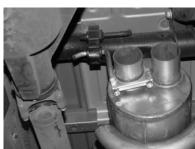
INSTALL MUFFLER #B ONTO HEADPIPE AT LEAST 1 ½" TO 2". USE CLAMP #F TO SECURE MUFFLER TO HEADPIPE. DO NOT TIGHTEN. USE A JACK STAND TO SUPPORT THE MUFFLER. OUTLETS SHOULD BE AT THE TOP. INSTALL HANGER #I ONTO DRIVERSIDE MUFFLER OUTLET AND INSERT WELDED HANGER INTO GROMMET. DO NOT TIGHTEN.
