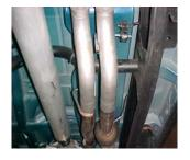
Install driverside headpipe #B onto factory pipe.
