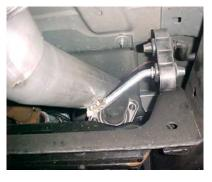
BOLT HEADPIPE # A ONTO YOUR EXISTING STOCK FRONT PIPE RE-USING FACTORY BOLTS. INSERT WELDED HANGER INTO RUBBER GROMMET.
