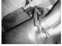
Install rear muffler hanger #H. Onto driver side outlet of the muffler, insert hanger into rubber grommet.
