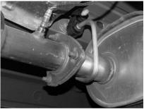
Lay out the exhaust on the floor so it looks like the drawing and compare the parts with the manual. To remove the stock exhaust, un-bolt it from the 3-bolt flange located in front of the muffler. **NOTE: For an easy removal of the exhaust, cut the tailpipe off behind the muffler.** Leave all rubber grommets in place. Use WD-40 to aid in removal.
