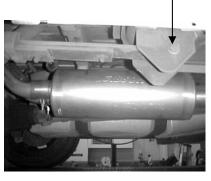
Install muffler #B onto head-pipe #A 1-1/2" to 2" with the louvers in the muffler facing towards the converter. Use a jack stand to support the muffler. Use Clamp #G to secure the muffler to the head-pipe. **Do Not Tighten at this Time!**
