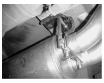
Install rear muffler hanger #H.
