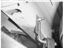
Install tailpipe hanger #J on the frame, then measure 9" from the rear; you will see a 1" round hole use this to mount your hanger. Use the bolt kit and rubber grommet provided in your kit, # K & L
