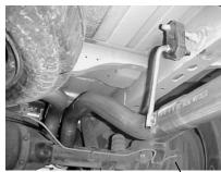
Install the Passenger side over-axle tailpipe # C to the muffler, 1-1/2" to 2". Insert welded hanger into rubber grommet. Use clamp # I secure the tailpipe to the muffler.
