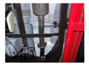
**4.** Install muffler #B onto head pipe #A 1½"-2". Use a jack stand to support the muffler. Use clamp #E to secure the muffler to the headpipe. Do not tighten.
