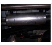
**3.** Install muffler #C onto headpipes 1½"-2" with the louvers facing towards the Y-pipe. Use a jack stand to support the muffler. Use clamp #G to secure the muffler to the headpipes. DO NOT TIGHTEN.
