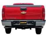
9. Install stainless steel tip. Clamp down. When you have everything in place, firmly tighten all bolts and clamps down securely. Use stainless steel cleaner and a Scotch Brite pad weekly to prevent tip from discoloration. Inspect all fasteners after 25-50 miles of operation and re-tighten as necessary.
