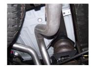
5. Slide the over axle tailpipe #C into the muffler 1.5-2". Use clamp #E to secure tailpipe to muffler. Do not tighten. Insert welded hangers into rubber arommets.
