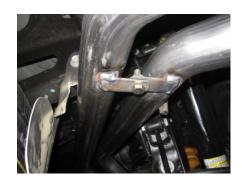
6.Once tailpipes are installed use bolt kit #H to secure pipes together the driver side tab will be on the bottom.
