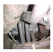
Install passenger side over axle tailpipe # C into muffler and attach using clamp # G. Insert welded hanger into rubber grommet. Use bolt kit # H to attach the tailpipes together.
