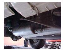
Install the driver side over axle tailpipe # D into the muffler. Use clamp # F to secure tailpipe to muffler. Do not tighten. Insert hanger into rubber grommet.
