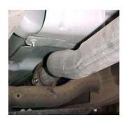
Lay out the exhaust on the floor so it looks like the drawing and compare parts with manual. To remove the stock exhaust un-bolt it from the flange located in front of the muffler. You will re-use your stock hardware.
