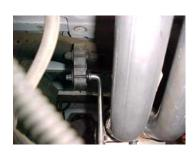
Install muffler # B onto head pipe 1-1/2" to 2" with the louvers facing towards the converter. Use a jack stand to support the muffler. Use clamp # G to secure the muffler to the head pipe. Do not tighten. Muffler inlet is looking into the louvers.
