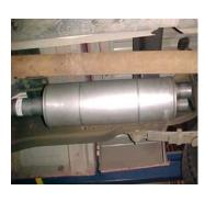
INSTALL MUFFLER AND ATTACH TO HEADPIPE. USING CLAMP #G. DO NOT TIGHTEN. USE JACKSTAND TO SUPPORT MUFFLER.
