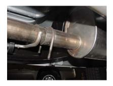
UNCLAMP THE STOCK **EXHAUST JUST IN** FRONT OF THE MUFFLER. YOU MAY NEED TO HEAT IT UP FOR EASIER REMOVAL. LEAVE ALL RUBBER GROMMETS IN PLACE. USE WD-40 TO AID IN REMOVAL OF EXHAUST AND HANGERS.
